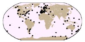
The ULR analysis center consortium was established in 2002 to process GPS data from stations at or close to tide gauges. It contributes to the TIGA pilot project since October 2002 by providing weekly solutions with 460 days latency. The data analysis is performed using: (i) GAMIT software (King and Bock 2005) for processing on a free network approach the GPS measurements that are split into several global clusters,
