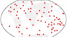
The Australian Universities analysis center consortium was established in 2002 initially to process GPS data from sites co-located with tide gauges only in the Australasian region. In 2007 we have commenced processing global data, using 2 x 40 station interwoven networks. The data analysis is performed using the GAMIT/GLOBK software (King and Bock, 2007; Herring, 2005).
