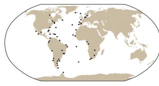
DGFI contributes to the TIGA project of the International GNSS Service (IGS) by operating permanent GPS stations at six tide gauges and by processing a network of about 60 GPS stations covering the entire North and South Atlantic Ocean. It contains also a few sites along the Pacific Ocean coastline, where the vertical datum of some Latin American countries is realized. In addition to the coastal sites, a number of IGS global stations are included in order to improve
